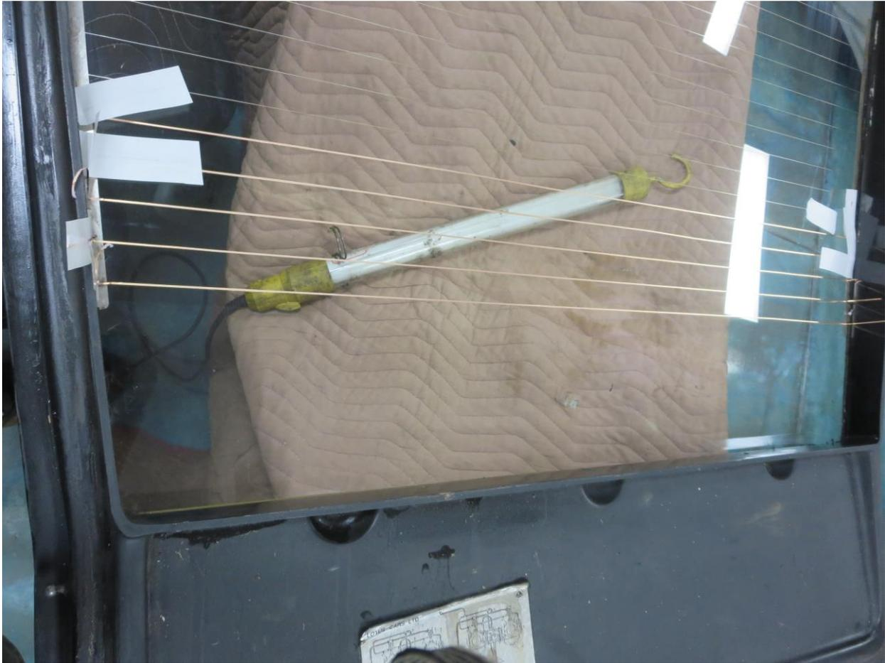
Once you have all the grid lines down, you then put the foam strip on the glass, then the copper buss bar, and fold the copper strips over this buss bar. Since just one side of each strip is conductive, they make contact with the buss bar. There is then a plastic cover placed over the buss bar to protect it from accidentally shorting.
