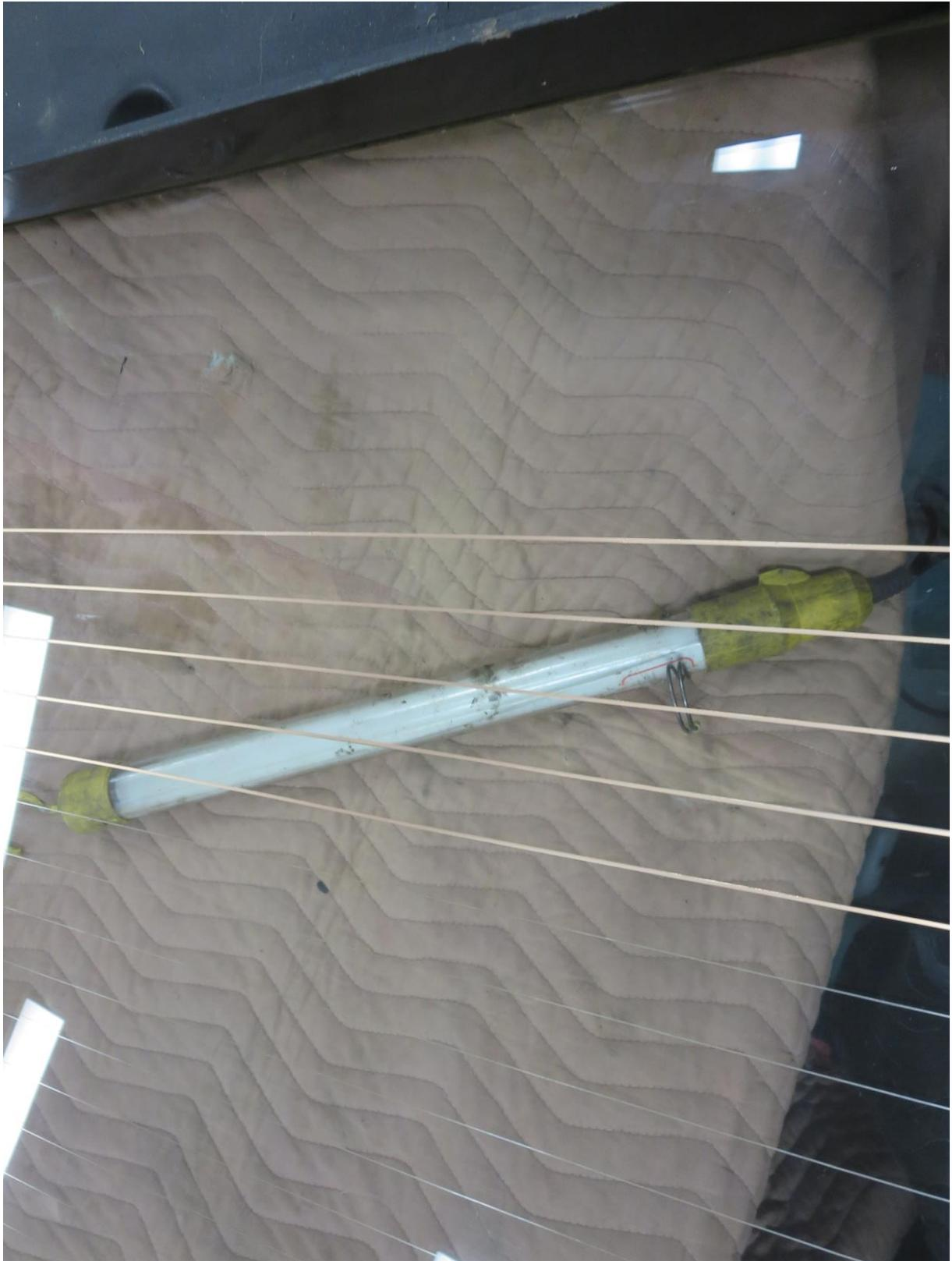
What you are left with are pieces of the copper strip hanging over the glass. The bottom of this strip is stuck to the glass, and the top side is copper, which is conductive.
